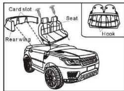
8. Assemble the empennage and seat cushion buckle into the body correspon ding to the position, fix the snap with the neck on the car body, then fasten by reoccupy two self-tapping screws
